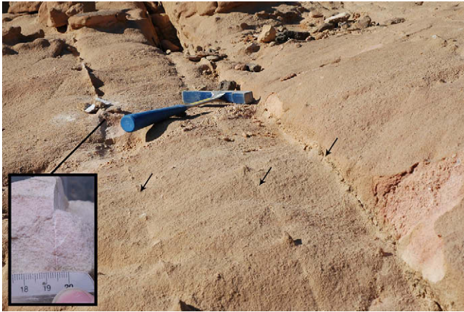
Fig. 4. Picture from the studied outcrop at locality 1 showing three individual deformation bands (indicated by arrows), all of which feature central slip planes. The inset shows a hand specimen taken from one of the deformation bands, where the slip plane is clearly visible. The scale bar on the inset is in centimetres.
